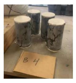
Fig. 2 76 mm x 152 mm UHPC cylinders
