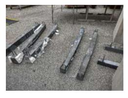
Fig. 5 Curved UHPC beams after form removal
