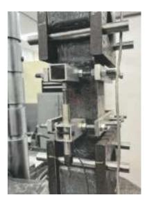
Fig. 3 Direction tension test
